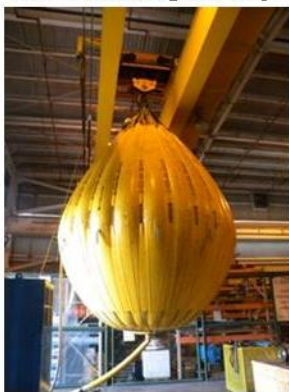
25te Warehouse crane (with flow meter and short rigging)
